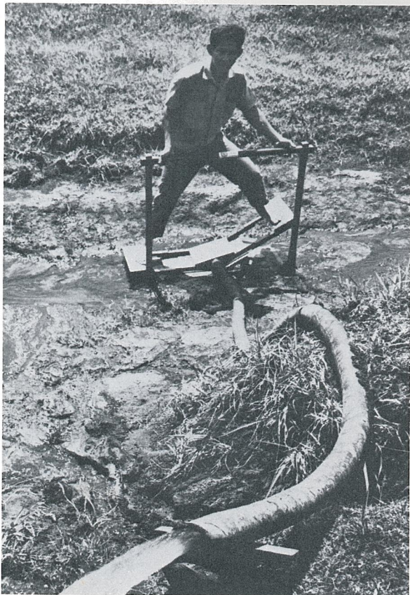
Figure 2-16 Foot-operated diaphragm pump developed by the International Rice Research Institute
