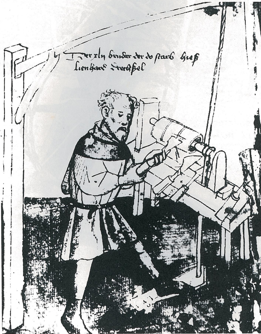
Figure 1-18 Foot-powered lathe (Courtesy of Friedrich Klemm)
