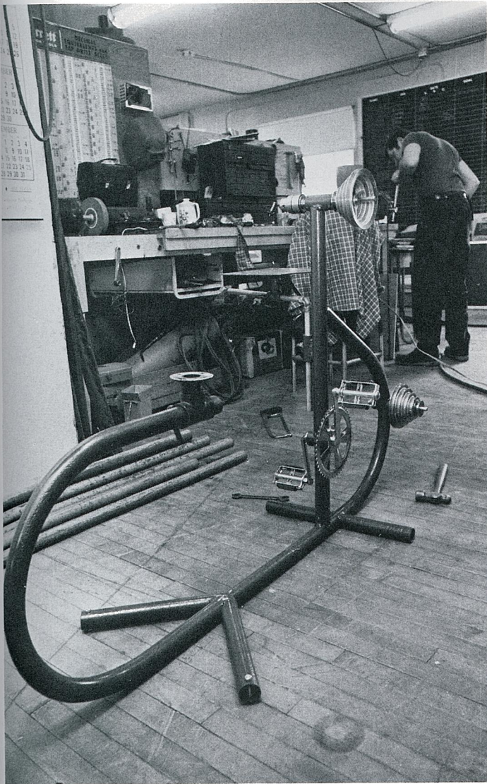
Figure 3-5 Streamlining of the cycle frame to cut down materials, weight, and width without loss of stability
