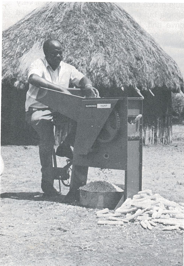
Figure 2-13 Commercial maize sheller in use in a village in Africa (Courtesy of Ransomes Sims & Jefferies Ltd., Ipswich, England)
